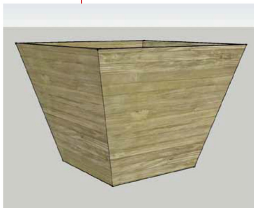
Two 1000 x 1000mm square top steel framed oak planters. 700mm high planted with large shrubs.
